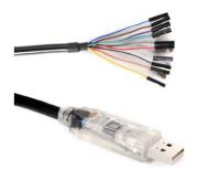
Figure 8.74 FTDI USB to MPSSE cable
