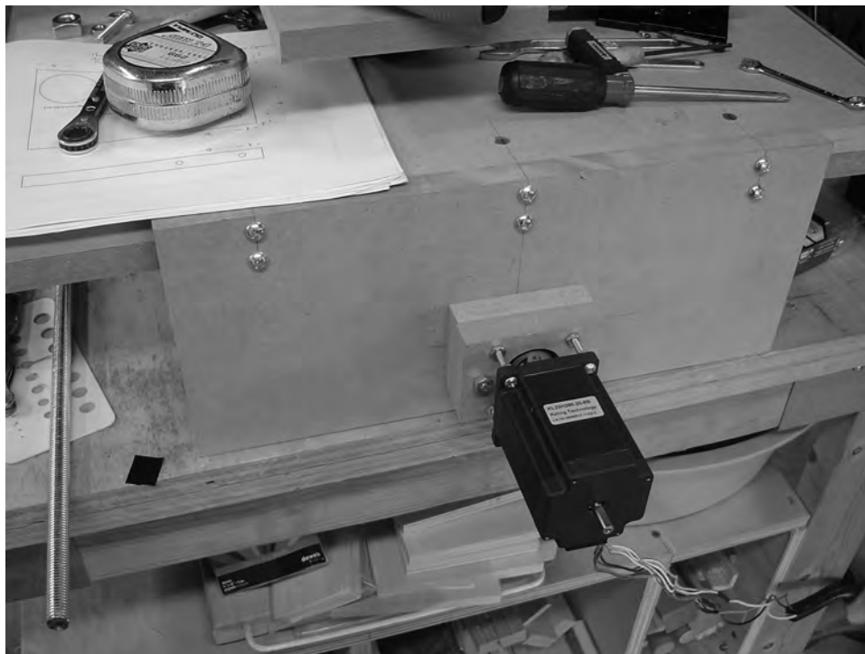
Figure 17-10. The x-axis leg has its motor attached.
