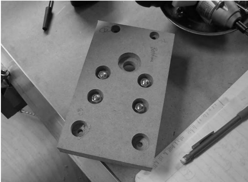
Figure 13-10. Drilling the lead screw bearing hole in Part D
