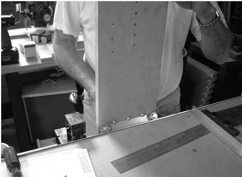
Figure 11-3. A single gantry side with a BRA rolling along the table's rail
