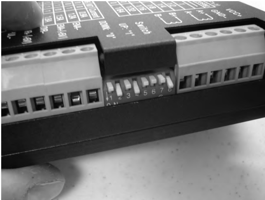
Figure 6-26. Configure the dip switches on each stepper motor driver.
