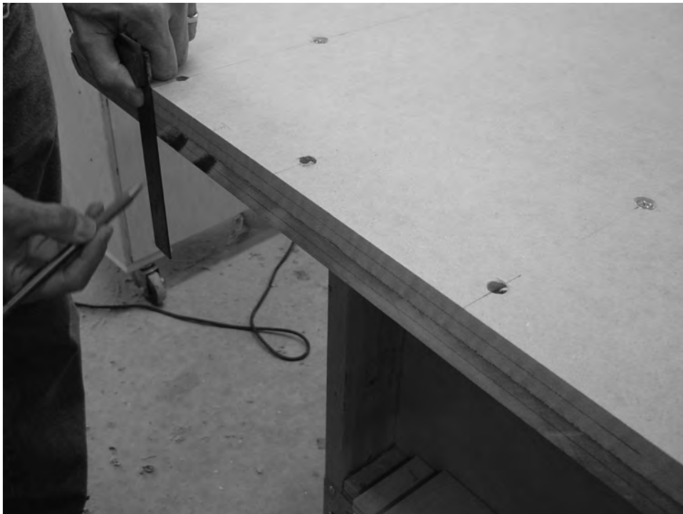
Figure 8-6. The tabletop with chamfered edges as seen from the end
