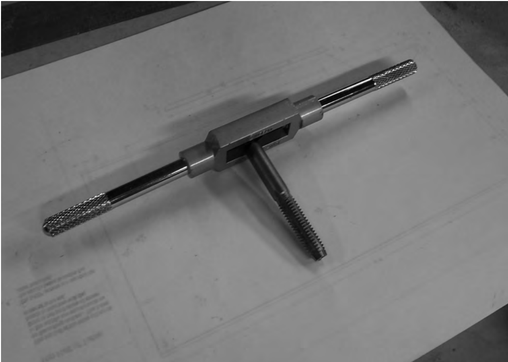
Figure 2-4. A tapping bit cuts threads into the aluminum angled rail.
