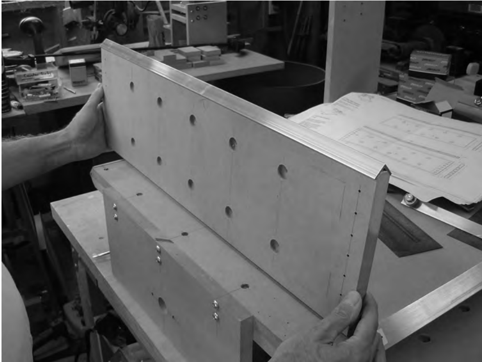
Figure 12-11. Cut two pieces of rail to be bolted to the top and bottom of Part O.
