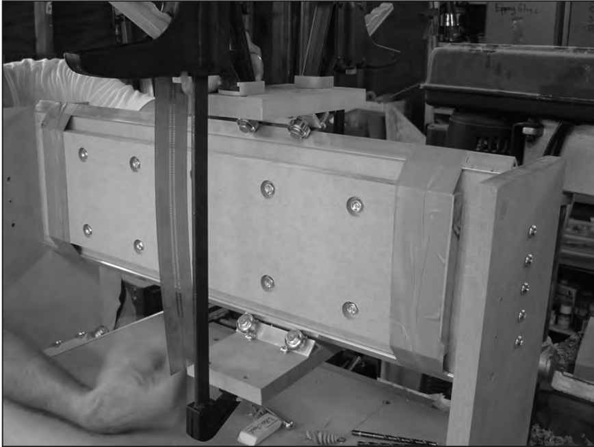
Figure 13-15. Clamp Parts C and D to the rail and measure the distance.
