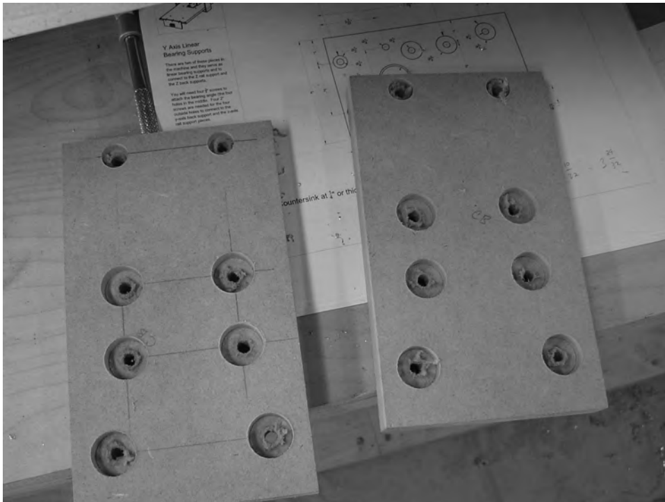
Figure 13-8. Counterbored holes with 1/4" drilled centers
