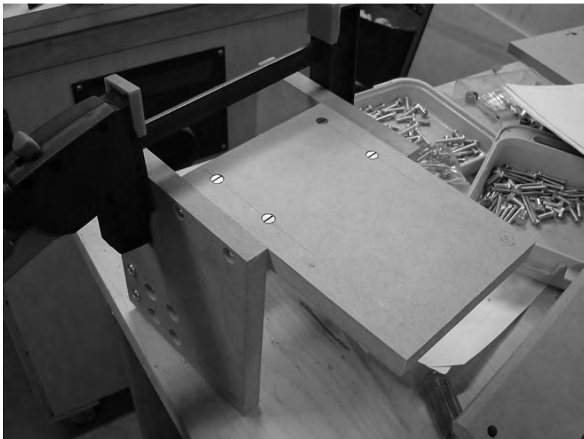
Figure 16-13. Use bolts and cross dowels to secure Part V to the z-axis assembly.
