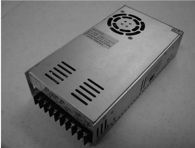
Figure 6-4. The power supply provides the proper voltage to all the electronics.
