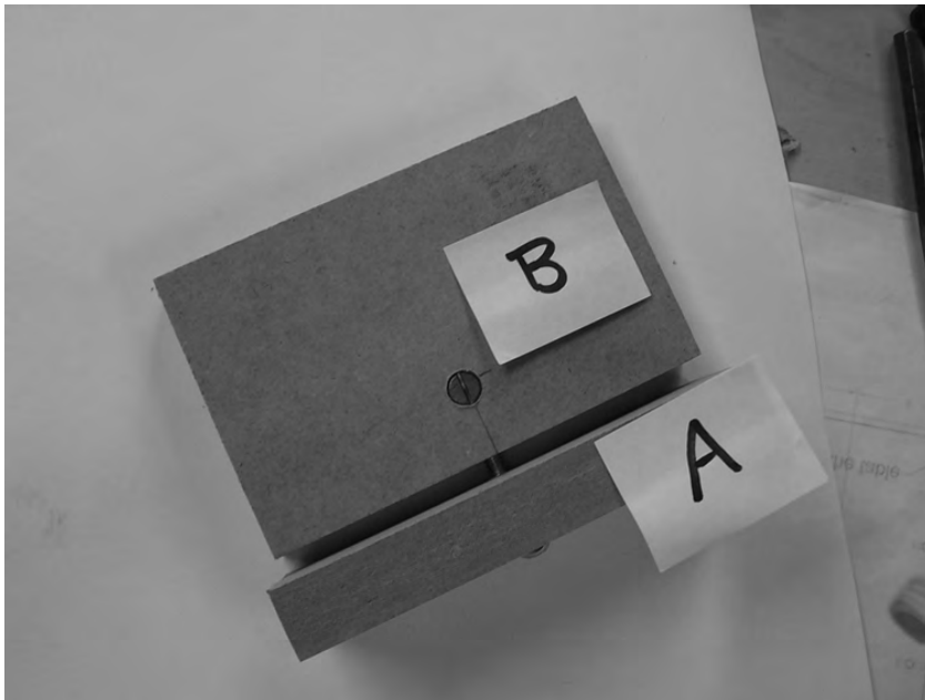
Figure 5-8. Align the 1/4" holes on Parts A and B and insert the cross dowel into the surface hole.
