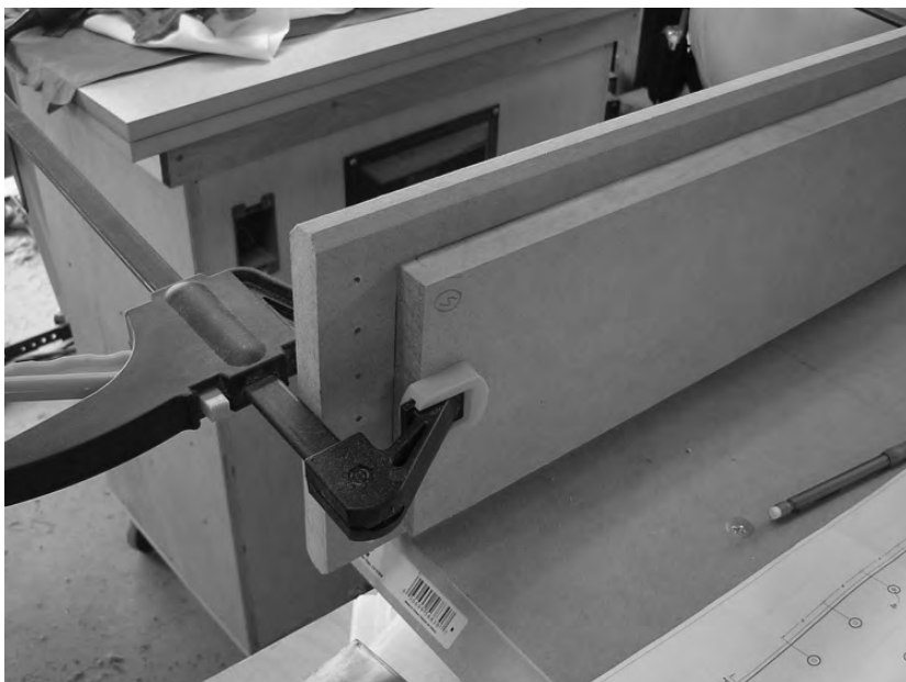
Figure 12-4. Parts O and S are clamped together for drilling.
