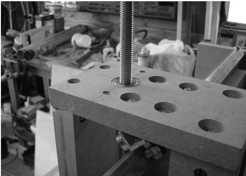
Figure 13-11. A piece of lead screw will go through the bearing inserted in Part C.
