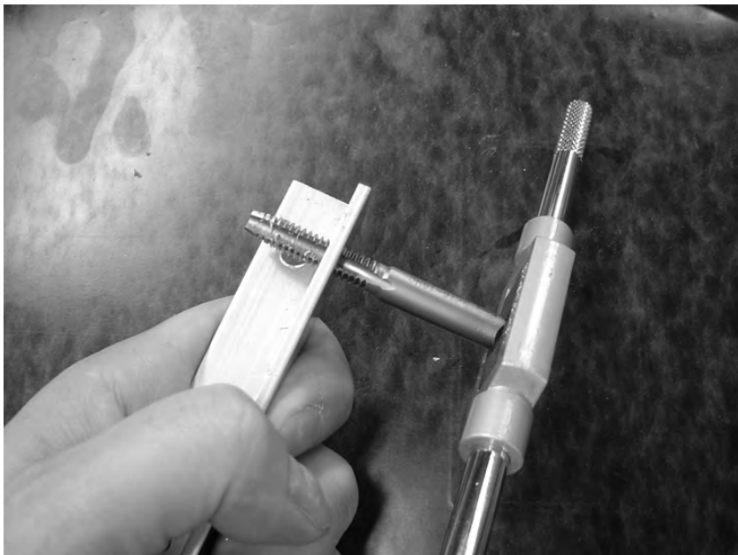
Figure 4-12. The tap bit over halfway through the hole
