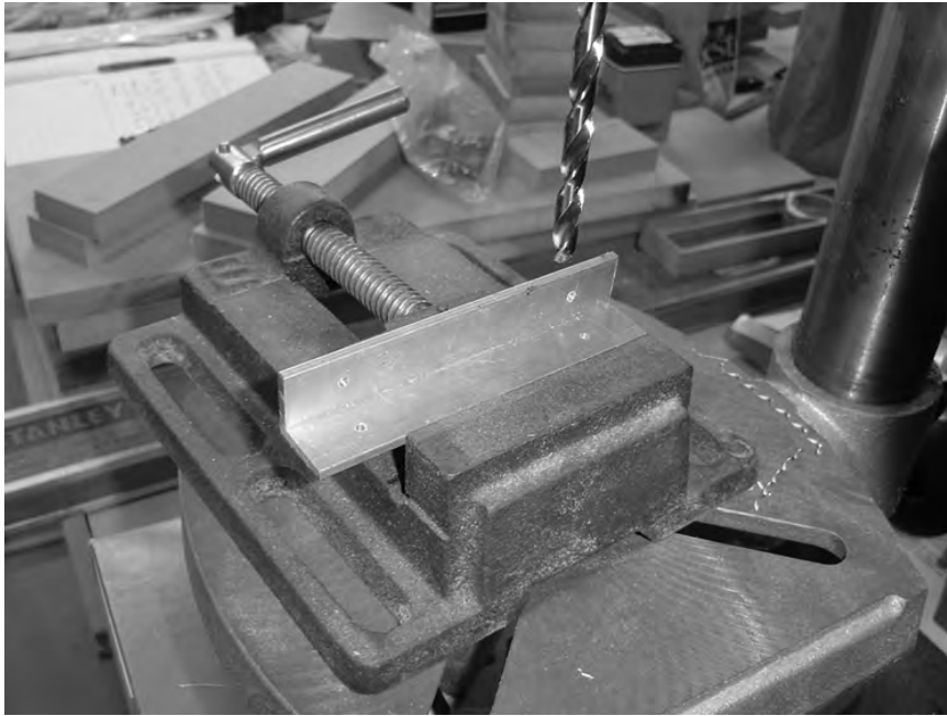
Figure 4-8. Four pilot holes drilled into a rail
