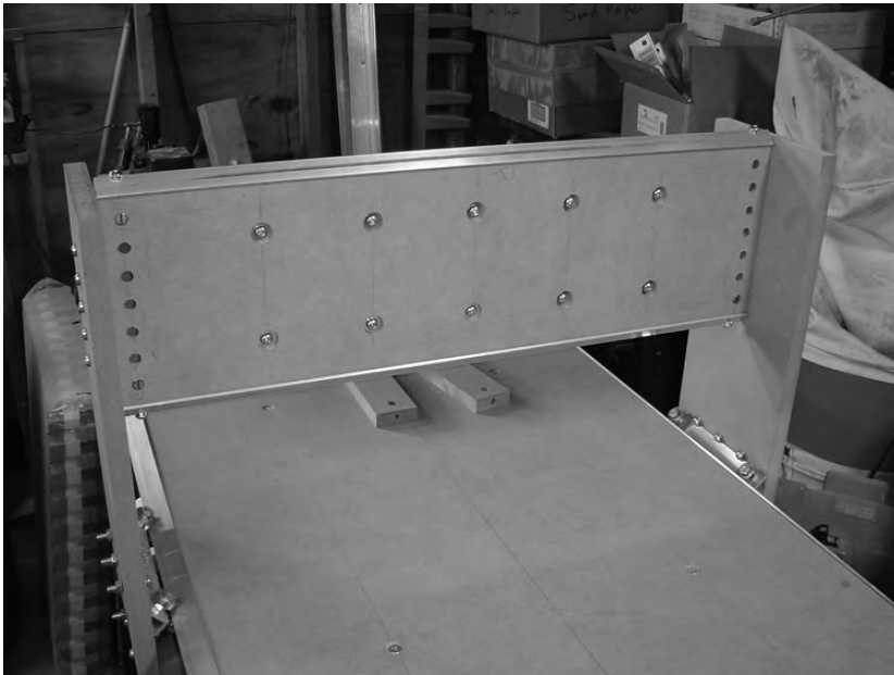
Figure 12-16. The aluminum rail drilled and bolted to the Y-Axis Rail Support (Part O).
