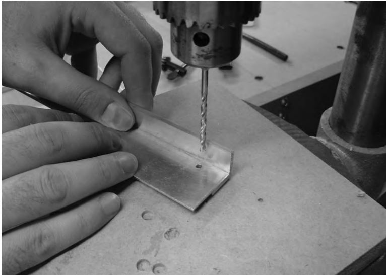
Figure 10-10. Drilling pilot holes into the BRA rails
