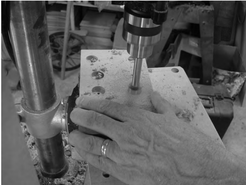
Figure 13-6. Drilling the counterbored holes in Part C
