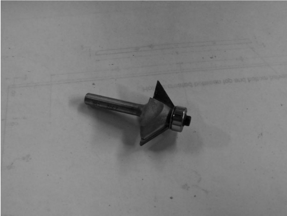
Figure 2-5. A chamfer bit will let you cut a 45 degree surface on the MDF.
