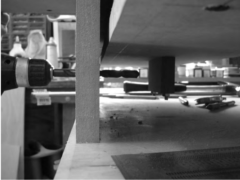
Figure 11-13. Drill a hole through Part E using a 1/2" drill bit.
