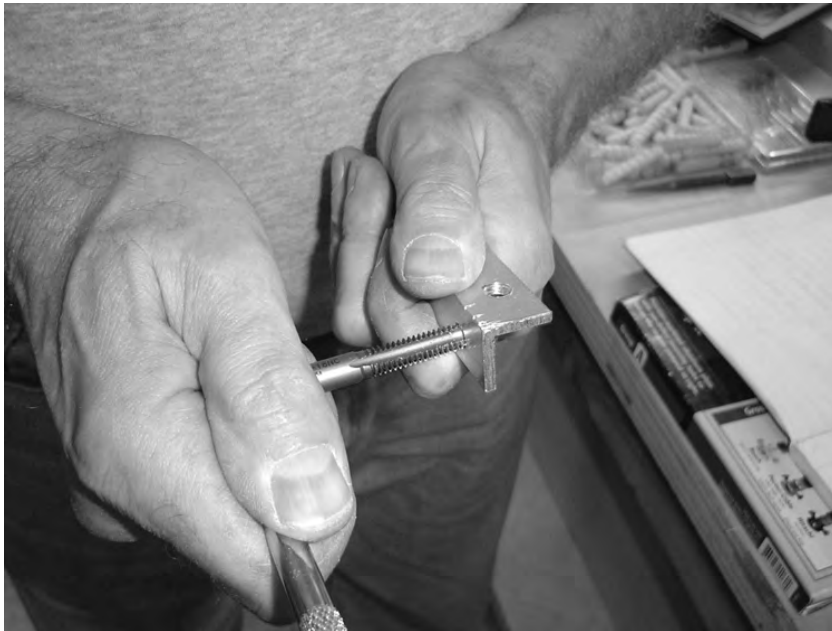
Figure 4-11. Cutting threads into one of the holes in the aluminum rail
