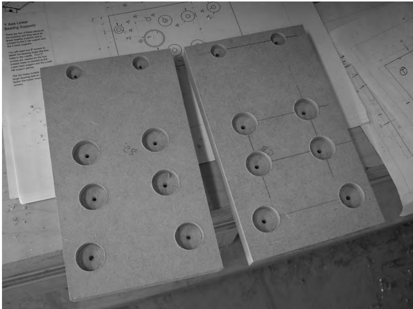
Figure 13-7. Parts C and D with counterbore holes drilled
