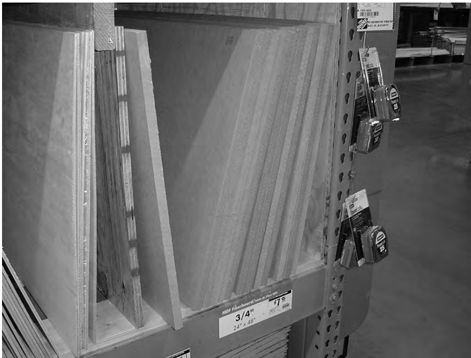
Figure 3-4. Try to find MDF in quarter-sheets with 2'×4' dimensions.
