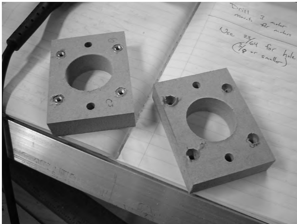
Figure 17-4. Counterbore four holes in the bottom motor mount for #8 nuts.
