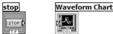
Figure 3.22. Your VI block diagram, showing the Stop Button and Waveform Chart terminals
