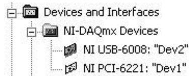
Figure 10.32. NI-DAQmx devices in MAX, showing the physical and simulated devices connected to your system
