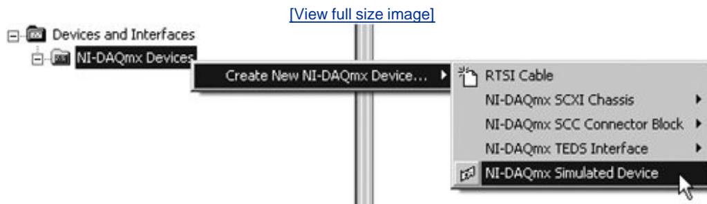
Figure 10.35. Creating a new NI -DAQmx Simulated Device in MAX
