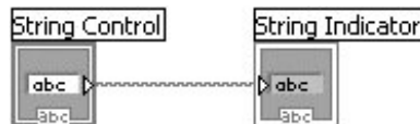
Figure 9.4. Block diagram showing that the string control passes its data, unchanged, to the string indicator
