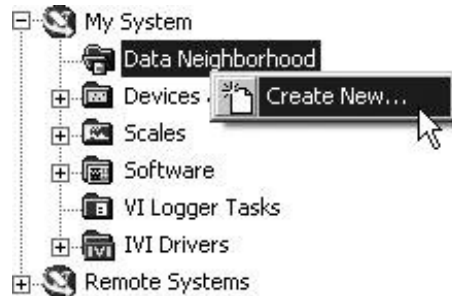
Figure 11.24. Launching the Create New . . . dialog from the Data Neighborhood node in MAX
