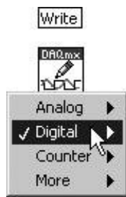
Figure 11.40. Write digital output
