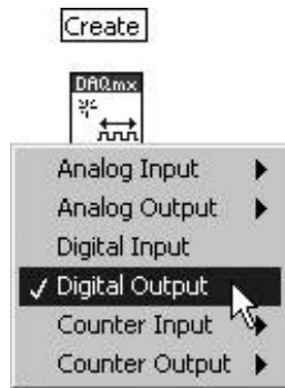
Figure 11.39. Create digital output task
