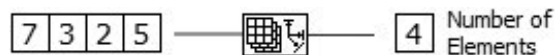
Figure 7.21. Array size used to determine the length of a four-element 1D array
