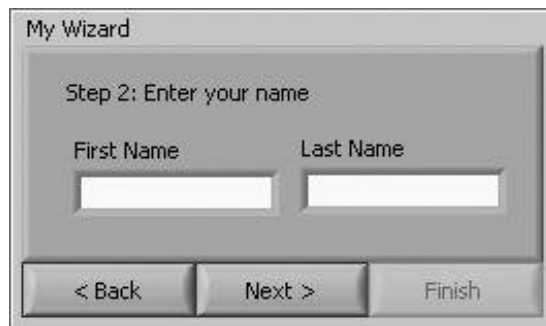
Figure 13.149. A "wizard" user interface created using a tab control with hidden tabs
