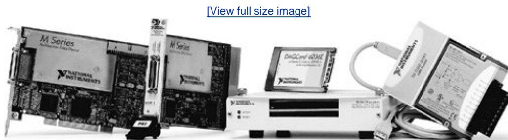
Figure 10.25. DAQ devices in a variety of form factors and bus types
