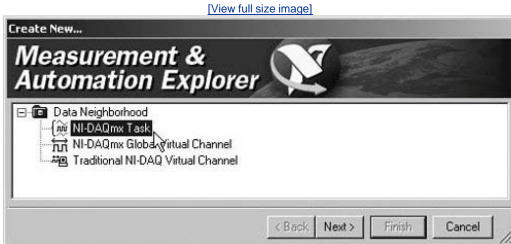
Figure 11.25. Selecting NI-DAQmx Task from the Create New . . . dialog
