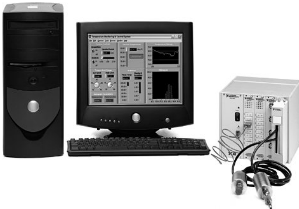
Figure 10.12. An SCXI chassis with several signal conditioning modules can be connected to a PC with LabVIEW.
