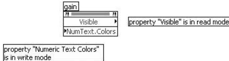
Figure 13.29. Property Node with Visible property in read mode and Numeric Text Colors in write mode
