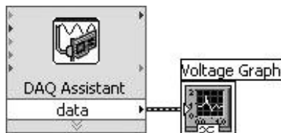
Figure 11.16. Buffered Analog In.vi using DAQ Assistant
