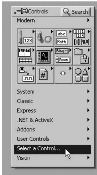
Figure 13.68. Choosing Select a Control . . . from the Controls palette to browse to a custom control file that you would like to add to the front panel
