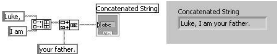
Figure 9.11. Using the Concatenate Strings function to build a sentence from a string and an array of strings
