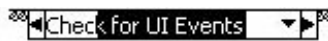
Figure 13.73. LabVIEW's auto-completion of case names as you type them into the Case Structure
