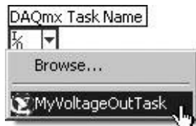
Figure 11.31. Selecting an NI-DAQmx task, created in MAX, from the DAQmx Task Name constant's drop-down list
