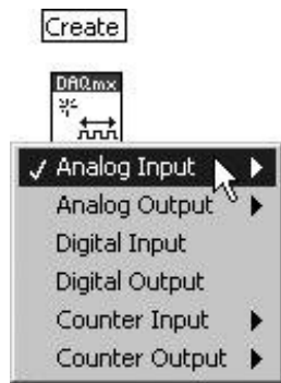
Figure 11.37. Create analog input task
