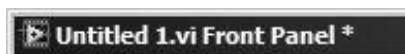
Figure 5.1. A VI window title with an asterisk (*) indicating that the VI has unsaved changes
