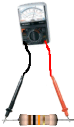
Fig 22. Resistance Measurement with Analogue Multimeter
