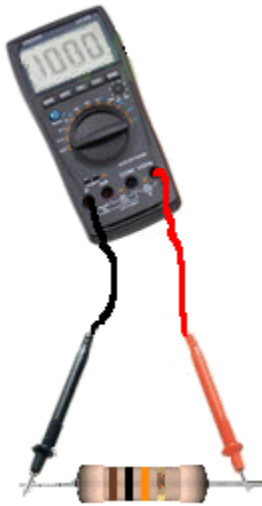
Fig 23. Resistance Measurement with a DMM
