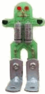
Fig 66. ROBOT MAN The ASTABLE MULTIVIBRATOR or "free-running" multivibrator.
