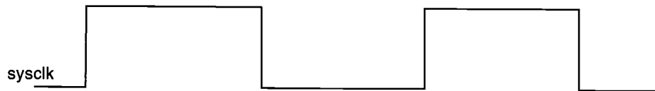
Figure D-4. A digital abstraction of the system clock signal.
