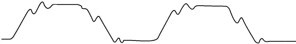
Figure D-3. An analog waveform for the system clock signal.
